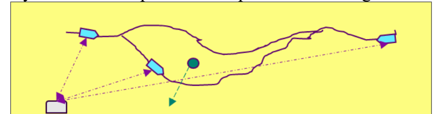
A mine SUT with three autonomous trucks controlled by a central computer. And a person is running.
